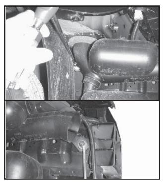
Remove air intake on passenger side, by removing one bolt and two plastic push fasteners.
